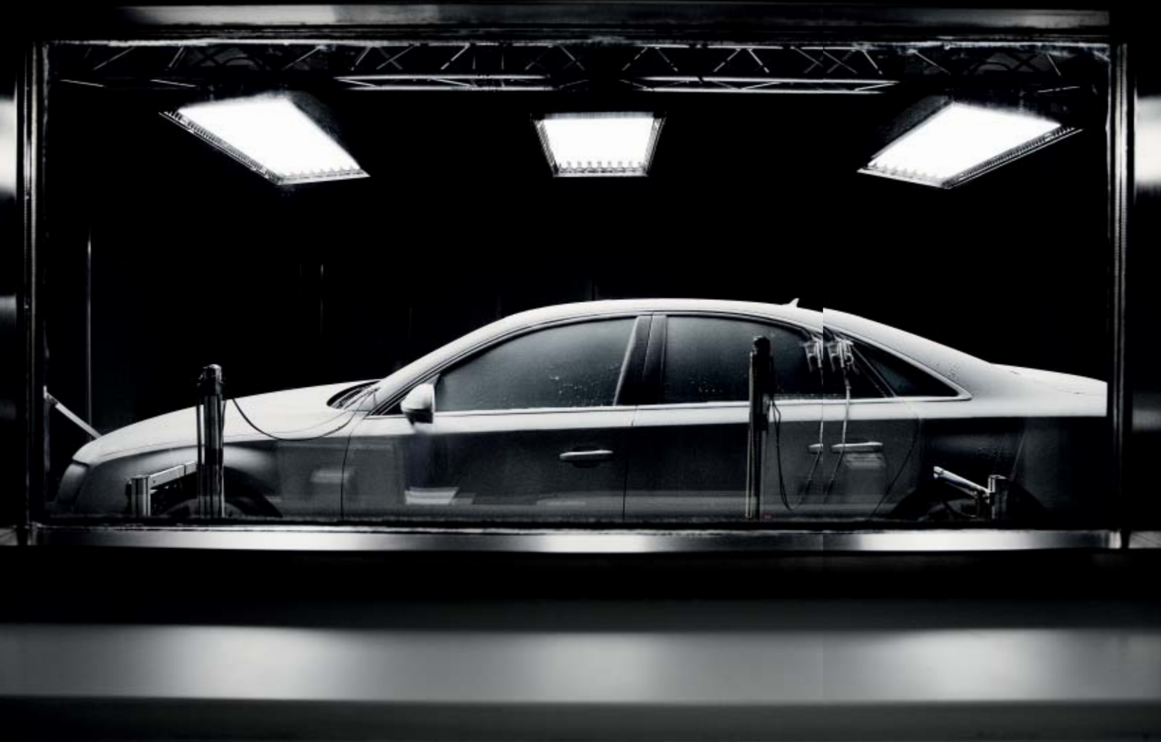
Climatic torture chamber: In the simulated weather tests, cars are first baked by artificial sunlight (02) and then frozen to minus 35 degrees (01).
