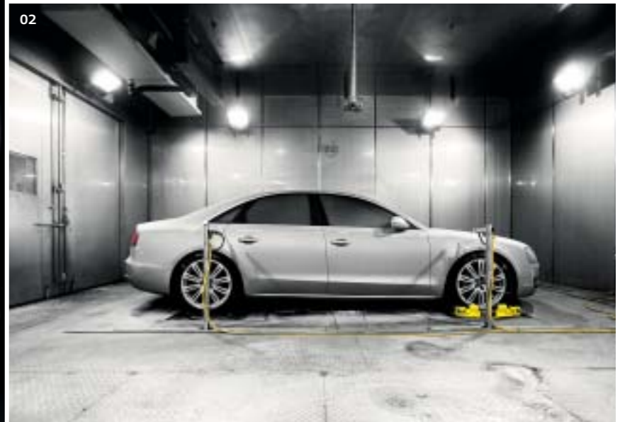
Climatic torture chamber: In the simulated weather tests, cars are first baked by artificial sunlight (02) and then frozen to minus 35 degrees (01).
